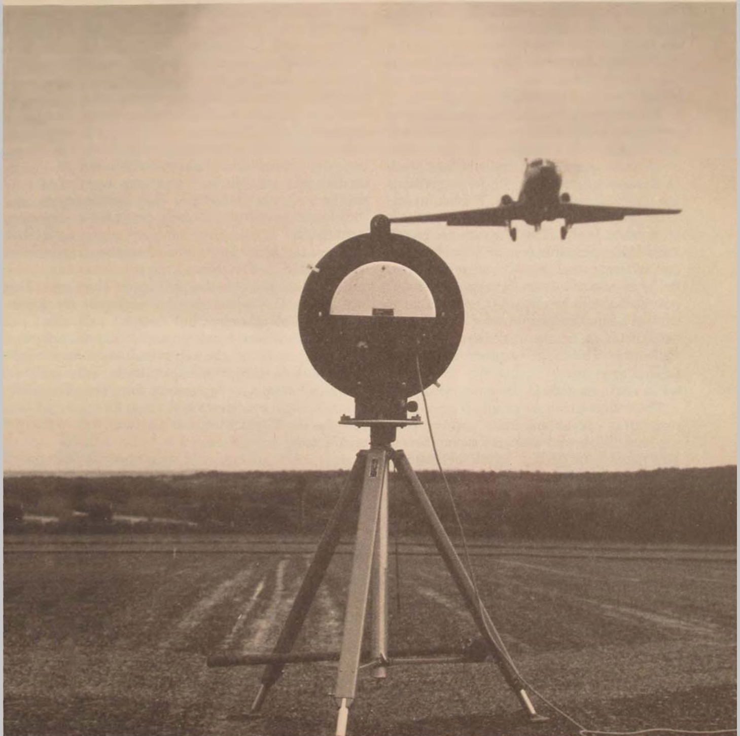
A T-39 approaching the Tactical Landing Approach Radar (TALAR) antenna. Investigation of pilot factors associated with advanced instrument technology is performed by R&D Division of the IFC.
